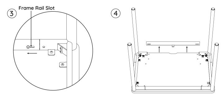
Grab the **Inside Base Screw** and slide the **Rail Connector** completely to the other side of the **Frame Rail Slot**. Repeat on the other side of the **Frame Rail**. Next, remove the **Frame Rail** from the **Desktop**. Keep the rails stored after removal as to not lose any components.
