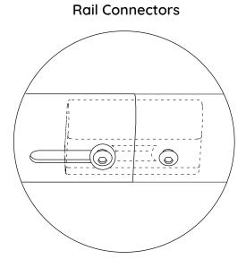
The Daily Desk uses modular **Frame Rails** with hidden **Rail Connectors**, one of which needs to be removed to install the **Cable Organizer**. Remove the **Rear Frame Rail** to install the Cable Organizer using the steps on the following pages.
