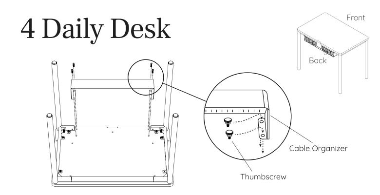
Position the **Cable Organizer** to the **Desktop** so that the open end faces the front of the **Desktop** as shown. Align the holes in the **Cable Organizer** to the threaded holes in the **Desktop** and tightly secure with the included **Thumbscrews** (x4).
