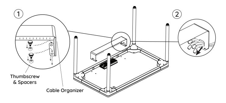
Position the **Cable Organizer** on to the underside of the **Desktop** so that the open end faces the front of the **Desktop** as shown. Align the holes in the **Cable Organizer** to the threaded holes in the **Desktop** and tightly secure with the **Thumbscrews** (x4) and **Spacers** (x4). Finally, route the Leg Cables through the top cutout tabs of the organizer.
