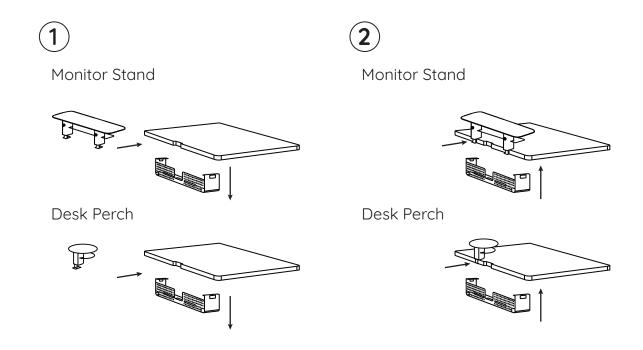
If you purchased a **Monitor Stand** or **Desk Perch**, prior to attaching, detach the **Cable Organizer** using the **Thumbscrews** (x4). Re-Attach the **Cable Organizer** with the **Thumbscrews** after **Monitor Stand** or **Desk Perch** Installation.
