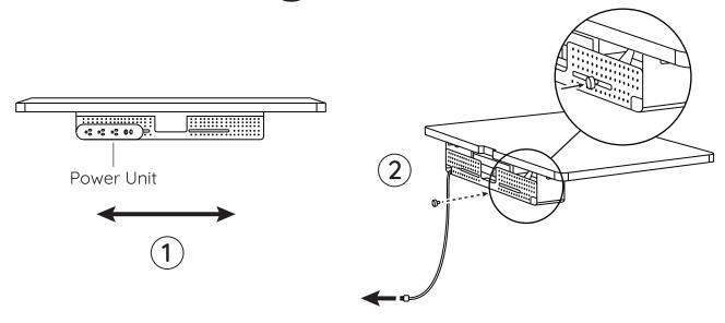
Install the **Power Unit** on the left or right side of the **Cable Organizer**. Depending on your setup, the Power Unit can be rotated so that the USB outlets are on the right or left side. Attach the Power Unit to the Cable Organizer using the **Thumb Screw** (x1). Note: the Thumb Screw fits into the adjustable slot of the Cable Organizer. Connect the **Power Cord** to the nearest outlet.
