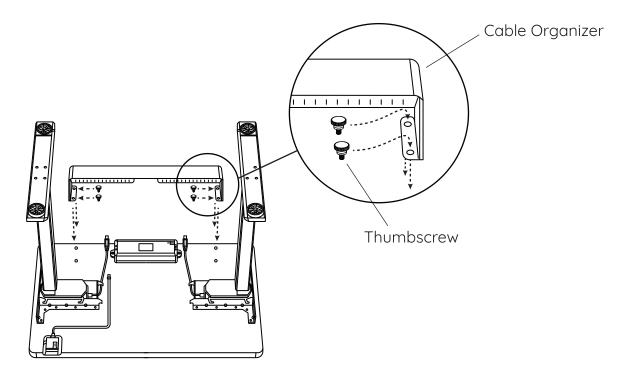
With your desk upside-down, position the **Cable Organizer** to the desktop so that the open end faces the front of the desktop as shown. Align the holes in the Cable Organizer to the threaded holes in the desktop and tightly secure with the **Thumb Screws** (x4).
