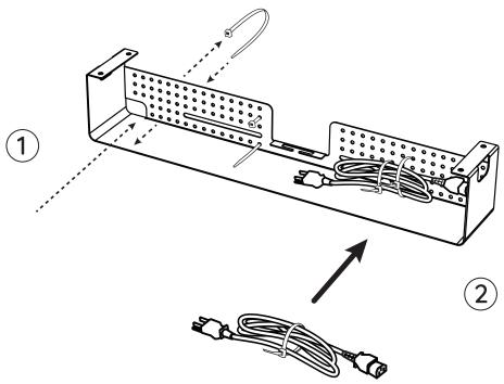
The back panel of the **Cable Organizer** has many holes for securing your cables and keeping your desk organized. For a tidy look, insert a **Cable Tie** (x8) through to the back of the **Cable Organizer** and then back to the front. Bundle and tie groups of cables together and then afix to the back panel using the pre-inserted Cable Tie. Repeat as needed.
