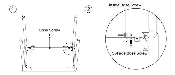
Using the **4mm Allen Key**, unscrew the **Base Screw** (x1) from the center of the rear facing **Frame Rail**. Next, unscrew and remove the outside **Base Screw** (x2) from the **Rail Connector**. Then loosen, but do not fully remove, the Inside **Base Screw** (x2) from the **Rail Connector**.
