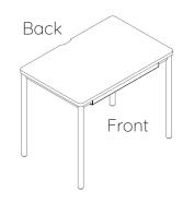
To install the optional **Desk Drawer**, First remove the **Front Frame Rail** (refer to steps 3 and 4).
