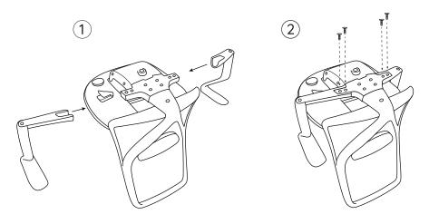
While the seat is still up-side down, insert the Armrests (x2) into both sides of the Bridge. Next, thread the Armrest Screws (x4), and tighten with the Allen Key.
